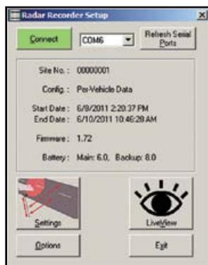
The buttons along the bottom of the screen are used to access other features of the setup which are discussed on the next few pages.
