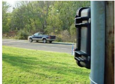
Again, note that it is the front of the Radar Recorder that you are aiming toward the road at a 45 degree angle.
