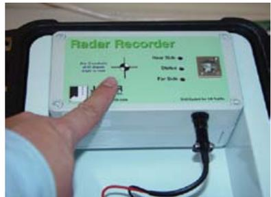
Second, check to see if there is anything between the Radar Recorder and the Road that may be obstructing the 'view' of the recorder.
