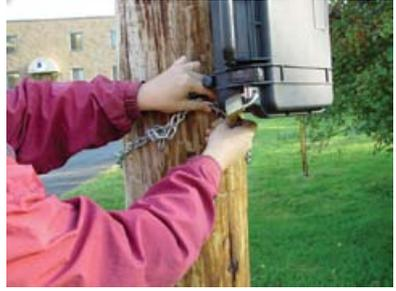
**Step #6** - Once the Radar Recorder has been setup using the TRAXPro software (refer to the next chapter), close the lid and lock it.
